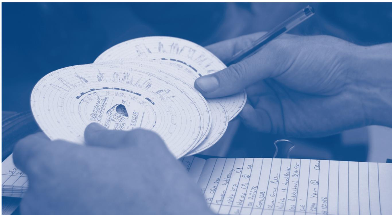
An approved tachograph is the required instrument by which the activity of drivers subject to the EU or AETR drivers' hours rules, and the vehicle's speed, distance and the time, are recorded. There are two main types of tachograph – analogue and digital.
